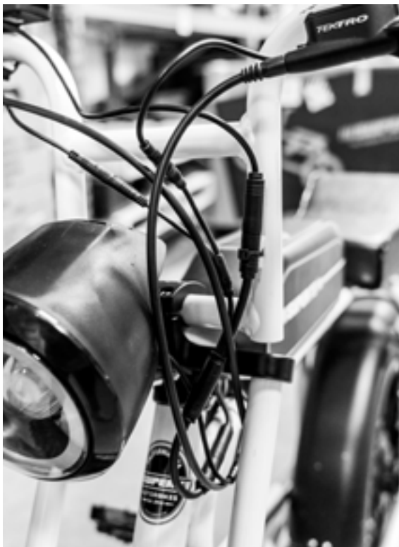
Proper configuration of cables with hydraulic brakes.
